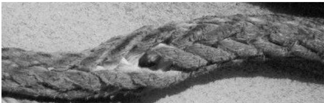
Figure 13 Inter-Strand Abrasion (Exposed internal core reveals wear)
