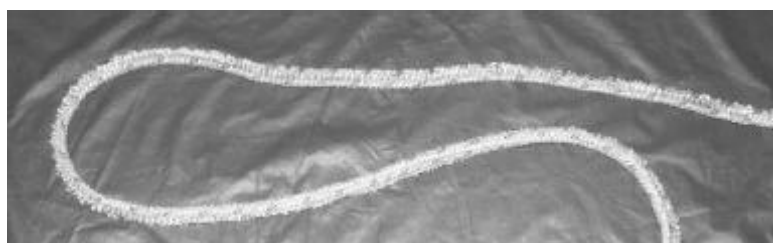
Figure 14 Uniform Surface Abrasion
