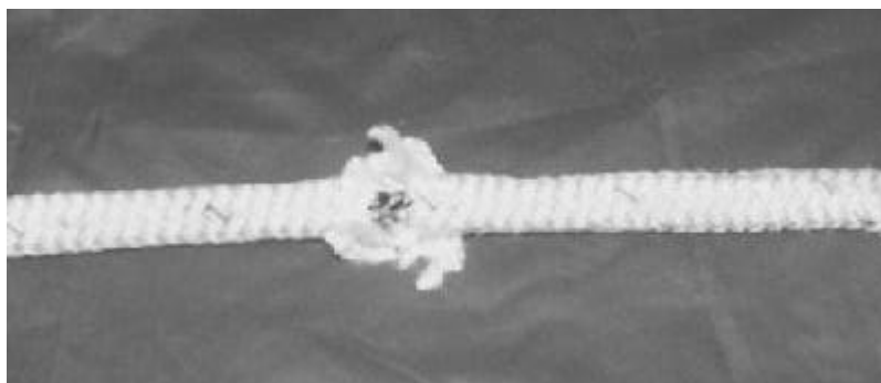
Figure 18 Cut in Jacket Exposing Core
